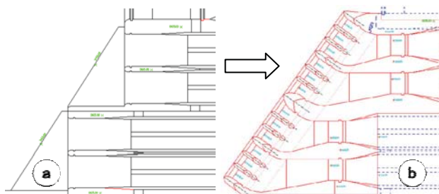
Figure 3: From initial (a) to the optimized (b) river intake design and transition to the desander basins.
